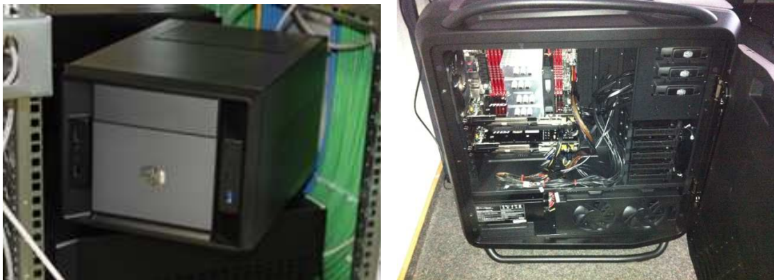
Figure II.8.: The two node types used in IGOR. The left picture shows very compact mini-ITX case with one discrete GPU, 16GB RAM and one HDD of 1TB. The right side depicts a large ATX tower with 64GB RAM, multiple GPUs and HDDs (8TB).
