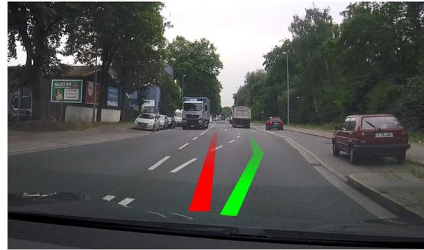
Fig. 14: Failure of expanding lanes. Red is the path the Tesla drove with Autopilot on, green is the path the Tesla should drive
