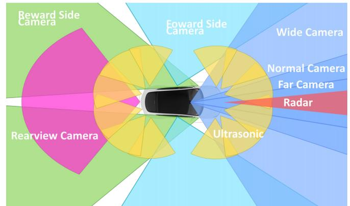
Fig. 4: Sensors at the Tesla Autopilot 2.0
