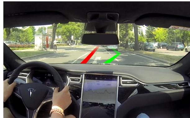
Fig. 15: Failure of merging lanes. Red is the path the Tesla drove with Autopilot on, green is the path the Tesla should drive
