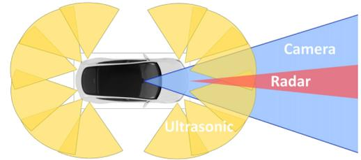
Fig. 3: Sensors at the Tesla Autopilot 1.0
